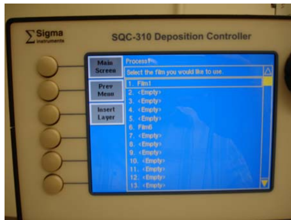
Figure 16: Add your film to the process you're building. Highlight the film of choice with the box and press Insert Layer .
