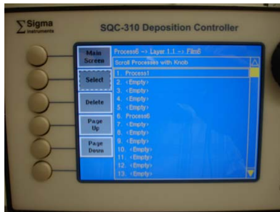
Figure 14: Process1 was created by pressing Create . That process is highlighted with the selection box and can be modified by pressing Select .
