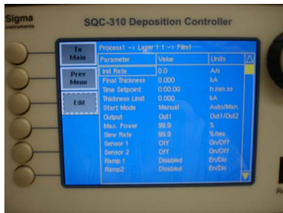
Figure 18: Define process parameters by highlighting with the scroll knob and pressing edit.
