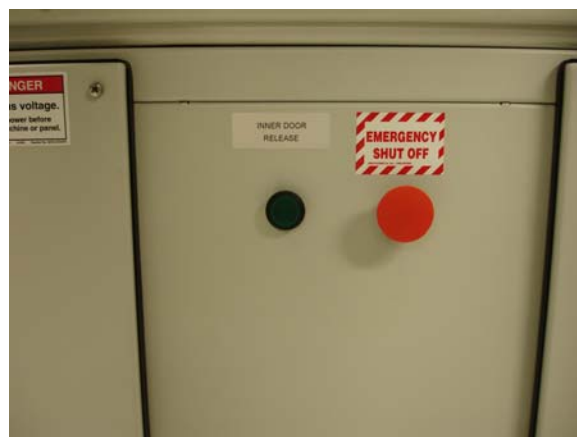
Figure 7: The evaporator door is operated from the front of the glovebox. Press “inner door release” to lock or unlock the vacuum chamber door.
