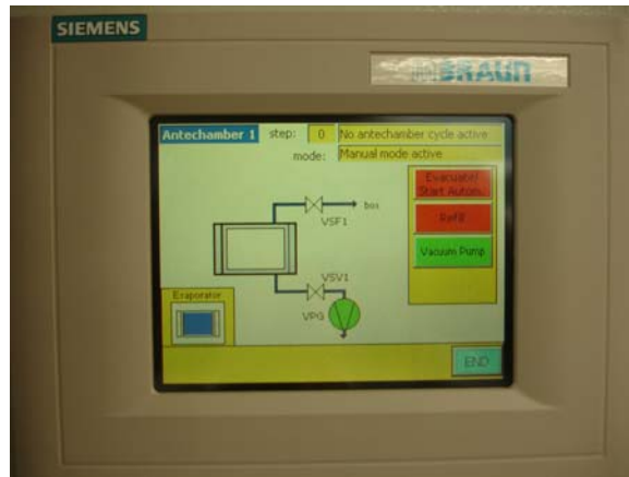
Figure 5: Antechamber 1 menu. The Evaporator button is located in the bottom left corner.
