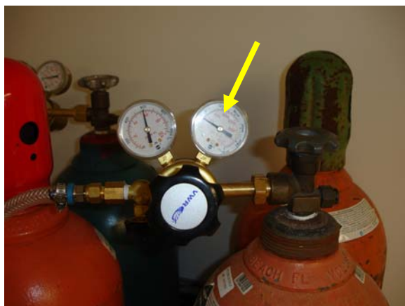
Figure 1: Read the N 2 cylinder pressure (dial indicated by yellow arrow) and record in logbook at start and end of glovebox use.
