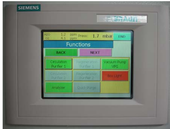
Figure 3: In the functions menu the Circulation Purifier 1 , Analyzer , and Box Light buttons are of importance.
