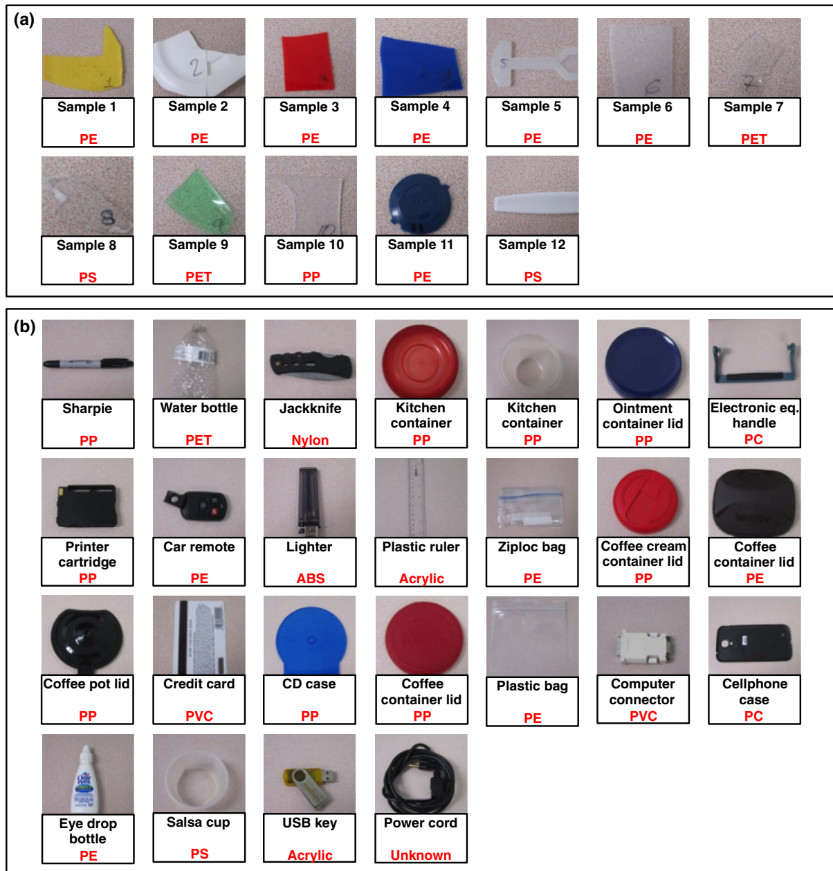
Fig. 7. Plastic samples randomly selected for the blind identification experiment based on the reported multi-spectral library. (a) Samples randomly picked from the characterized plastic batch used in experiment 1. (b) Plastic objects used in experiment 2.
